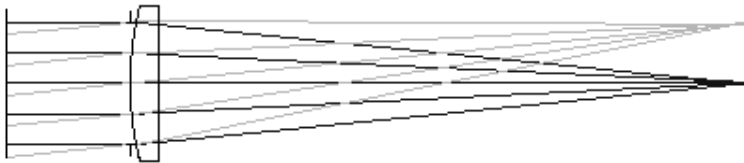
Figure 8.4 ZEMAX ray trace layout for f/5 plano-convex lens. Focal length (effective) = 100 mm, pupil diameter = 20 mm. Image positions are shown for 0 and 10 mm.
